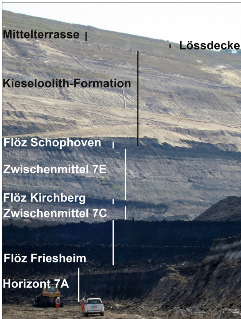
Text-fig. 7: Profile through the opencast mine Garzweiler. Layers near the Northern rim of the field (2015). Height about 180 meters
